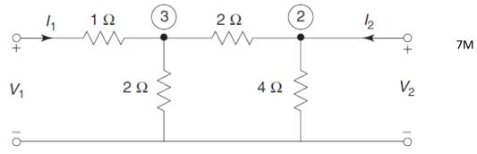
B) Two identical sections of the network shown in fig. are connected in cascade.Obtain the transmission parameters of the overall connection.
