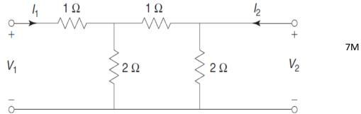
B) Determine Admittance(Y) parameters for the parallel connected networks shown in fig.
